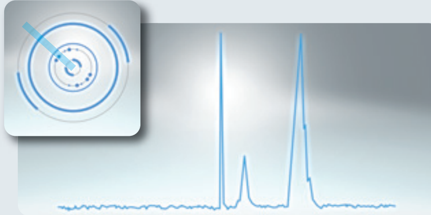
Theta/2Theta scan with 1-D detector, cut through Debye cones
