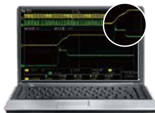
启动浪涌电流超电流量程，高速建立电压 (CV-High, CC-Low, CV优先)
