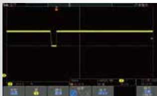
D/D Converter Sag Testing
